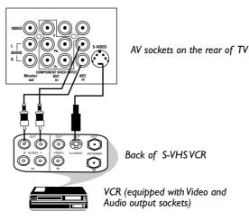
The S-Video connection on the rear of the TV is used for the playback of S-VHS VCR tapes, Video Discs, Video Games or Compact Disc-Interactive (cd-i) discs. Better picture detail and clarity is possible with the S-Video playback as compared to the picture from a normal antenna (RF) connection.
